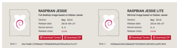
2. A new image can be downloaded at <https://www.raspberrypi.org/>. If you have put this image on your SD card and the raspberry has been started, log in with ssh from your desktop PC (also with Putty or any arbitrary terminal and enter **sudo raspi-config**).
